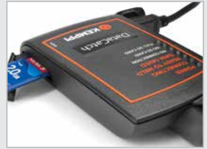
DataCatch device enables data collection
