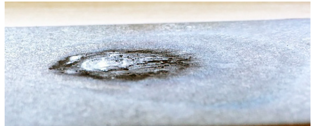
Spot weld removed
