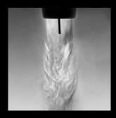
Shielding gas flow has a significant effect on weld quality. Normally shielding gas is invisible, but with Schlieren imaging technology it is possible to observe the real gas flow. This illustrates, how Flexlite GX welding gun design and consumable parts enable laminar gas flow and better shielding gas coverage.
