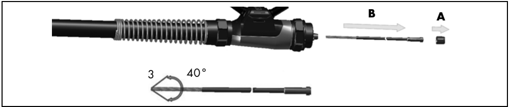
Fig. 3 Removing and deburring the liner
