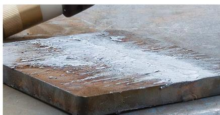
After the attachment is removed, operators can reduce the amperage on the system and wash any remaining material away without digging into the workpiece. FlushCut washing further reduces the need for grinding.
