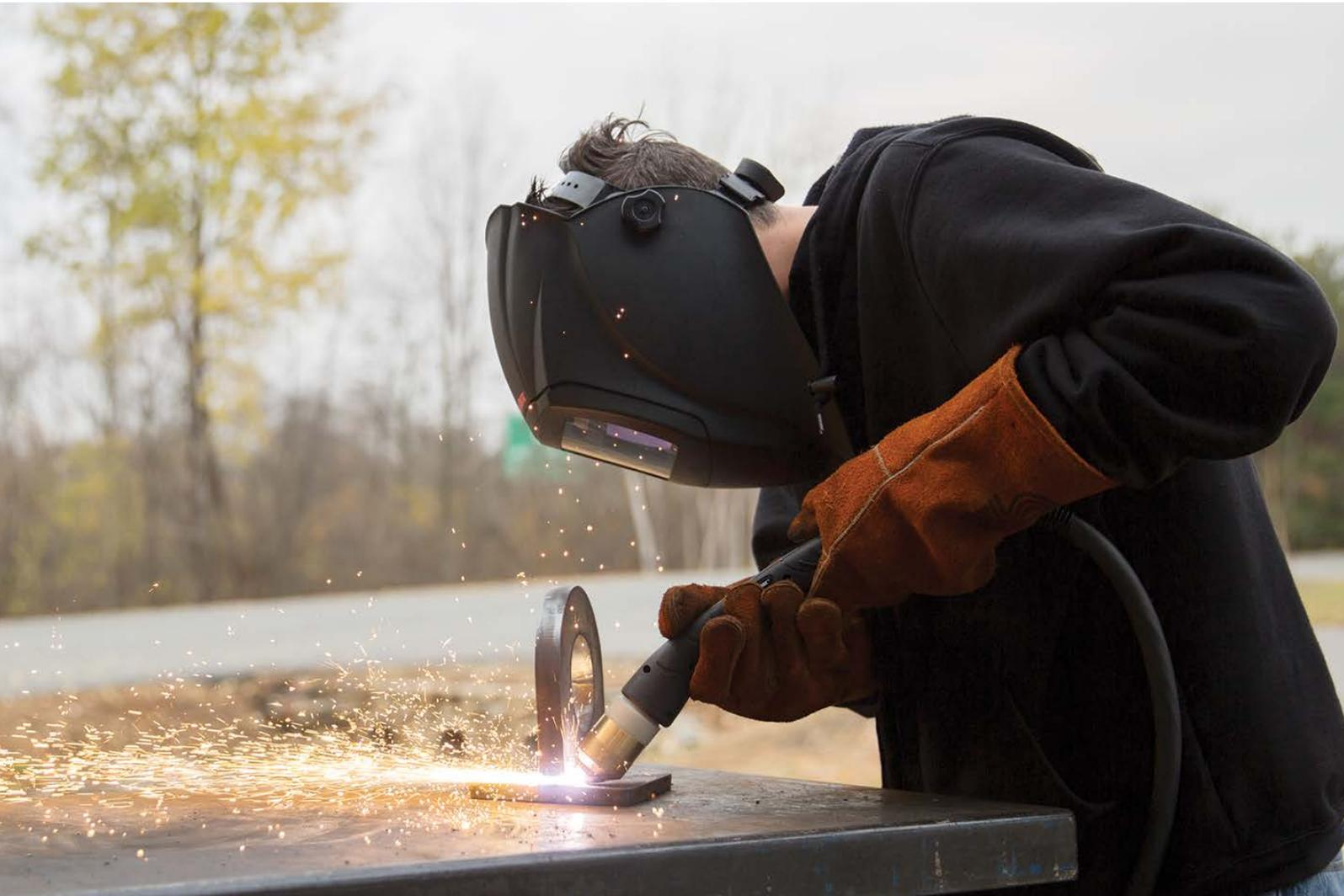
The FlushCut™ process for select Powermax systems provides users with the ability to cut closer to base materials than ever before.
