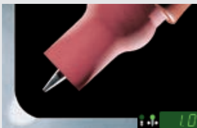
Cap diameter: 1 mm Base metal: AlMg3 Sheet thickness: 5 mm Welding amperage: 185 A Welding voltage: 15.6 V AC Balance: -5
