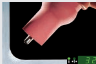
Cap diameter: 3.2 mm Base metal: AlMg3 Sheet thickness: 5 mm Welding amperage: 185 A Welding voltage: 15.6 V AC Balance: 0
