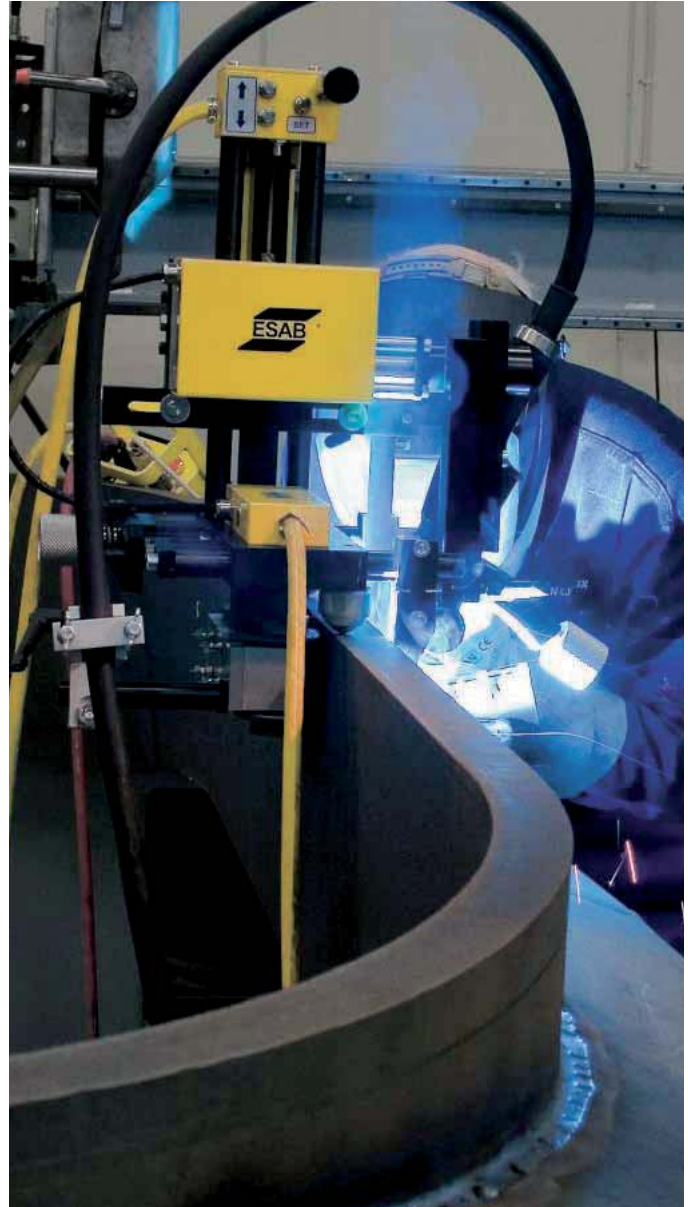
Frame 1 On this type of frame, the Frametrac can be used directly.
